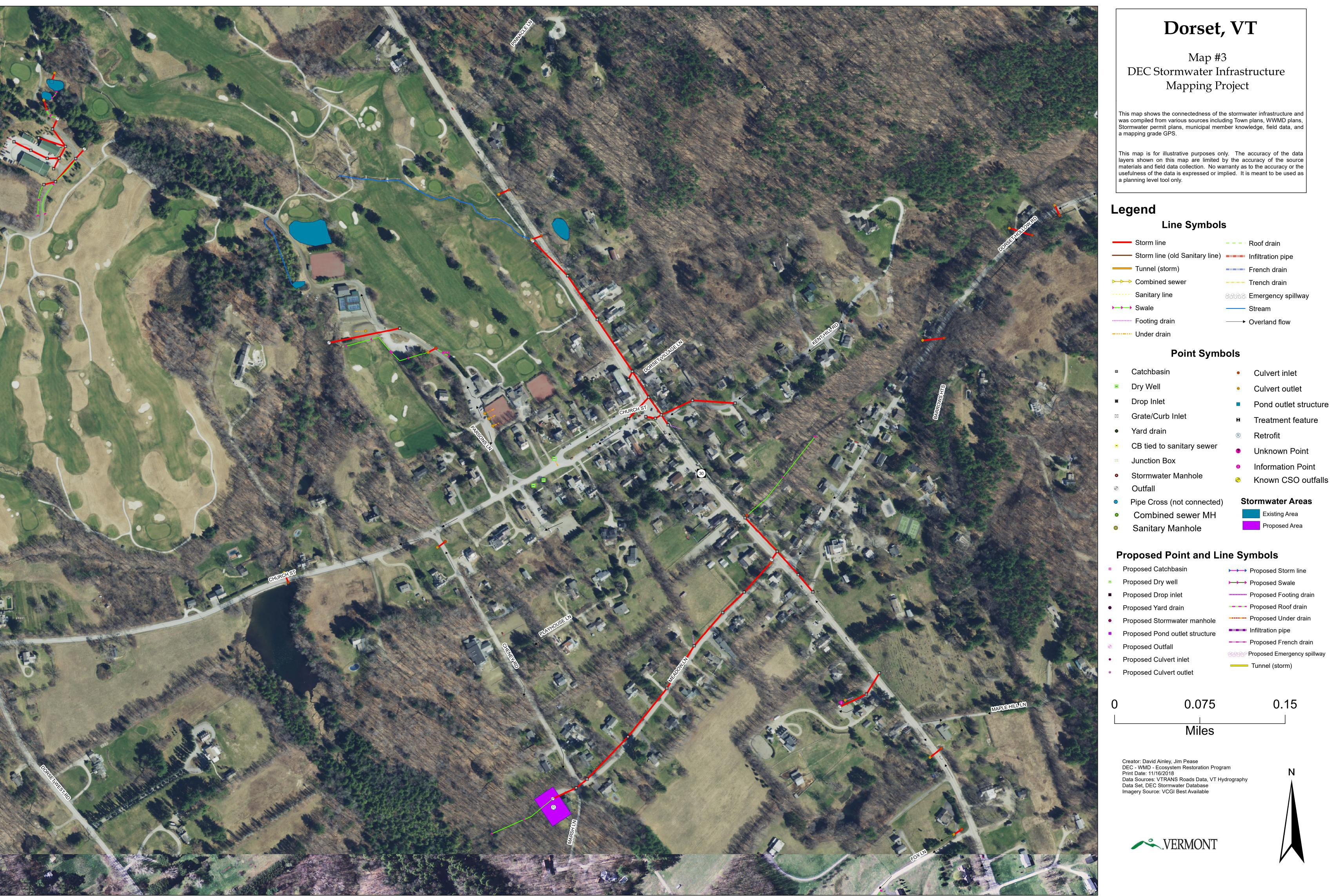
This map shows the connectedness of the stormwater infrastructure and was compiled from various sources including Town plans, WWMD plans, Stormwater permit plans, municipal member knowledge, field data, and a mapping grade GPS.
